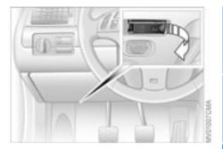
The interface socket for onboard diagnostics is located on the left-hand side of the driver's side, behind a specially marked cover located beneath the instrument panel. The cover has the letters OBD on it.
